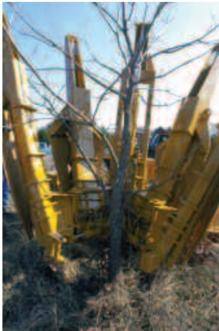
Left: The tree spade, used for transplanting trees and shrubs, can be used on riparian habitat projects, establishing turkey roost sites, and to create shrub thickets for quail and small game. Landowners renting this equipment will be provided an operator to run the machine.
