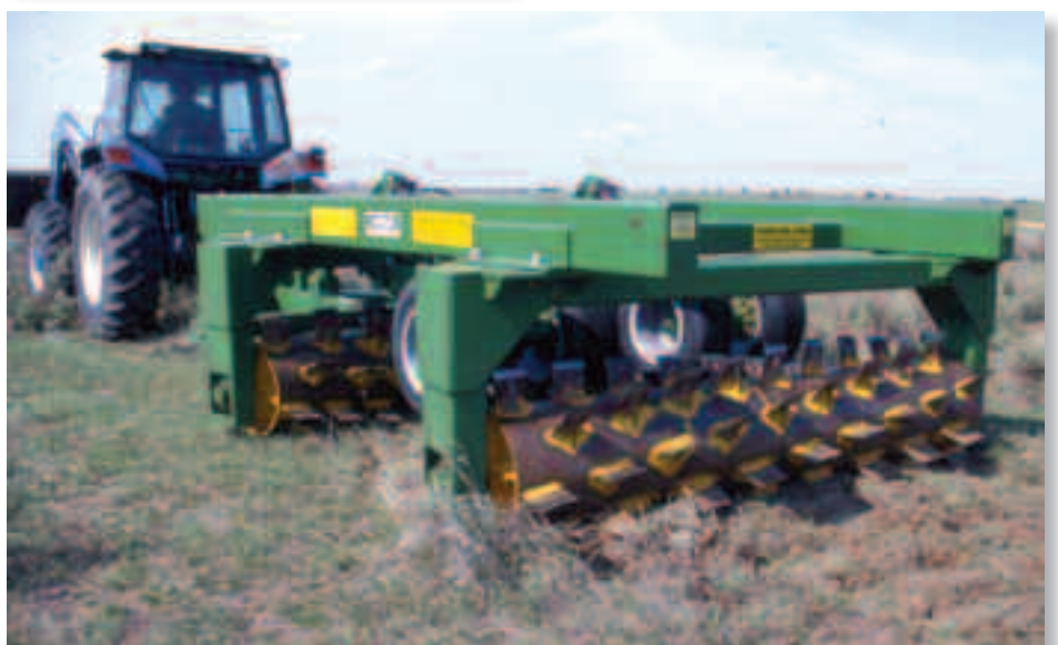
Below: Pulled behind a tractor, roller choppers crush and chop brush, small trees, and heavy plant growth. They also disturb the soil and allow sunlight and rain to reach the surface and encourage the growth of more desirable plants. A wide range of wildlife can benefit from this practice including quail, deer and turkeys.
