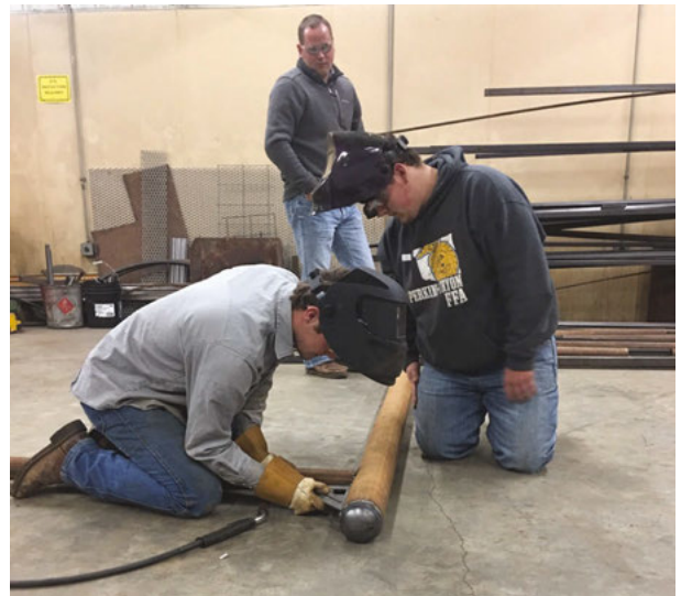
Members of the Perkins-Tryon FFA Chapter weld H braces in an effort to help rebuild miles of fences destroyed in wildfires in northwest Oklahoma. Courtesy photo.
