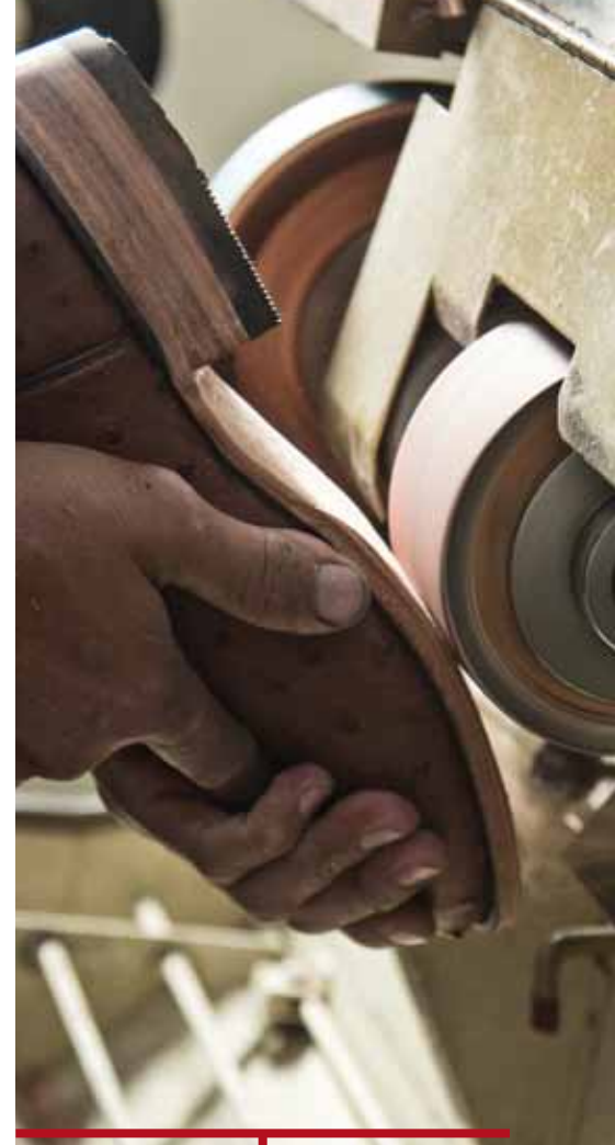
A worker sands the sole of a nearly finished boot in the Loveless shop.
